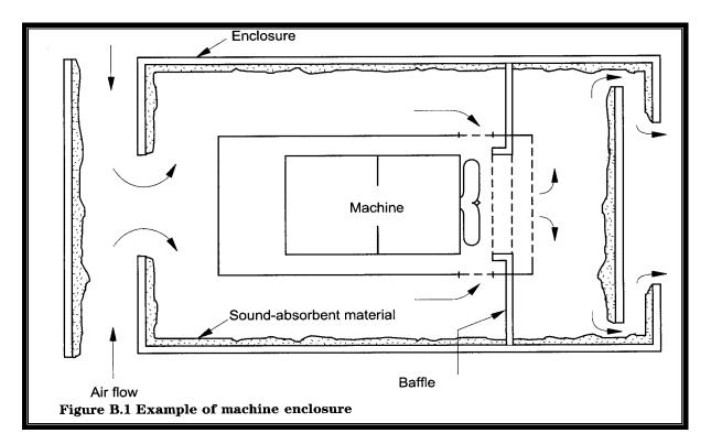
Figure 4.1a: Typical enclosures to reduce noise nuisance Reproduced with the permission of the British Standards Institution under licence number 2003SK/055.
