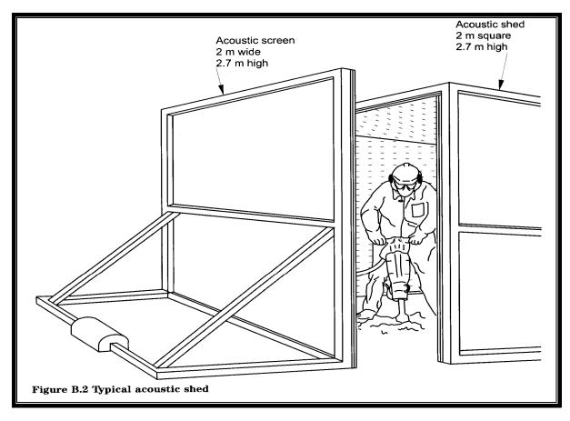
Figure 4.1b: Typical enclosures to reduce noise nuisance Reproduced with the permission of the British Standards Institution under licence number 2003SK/055
