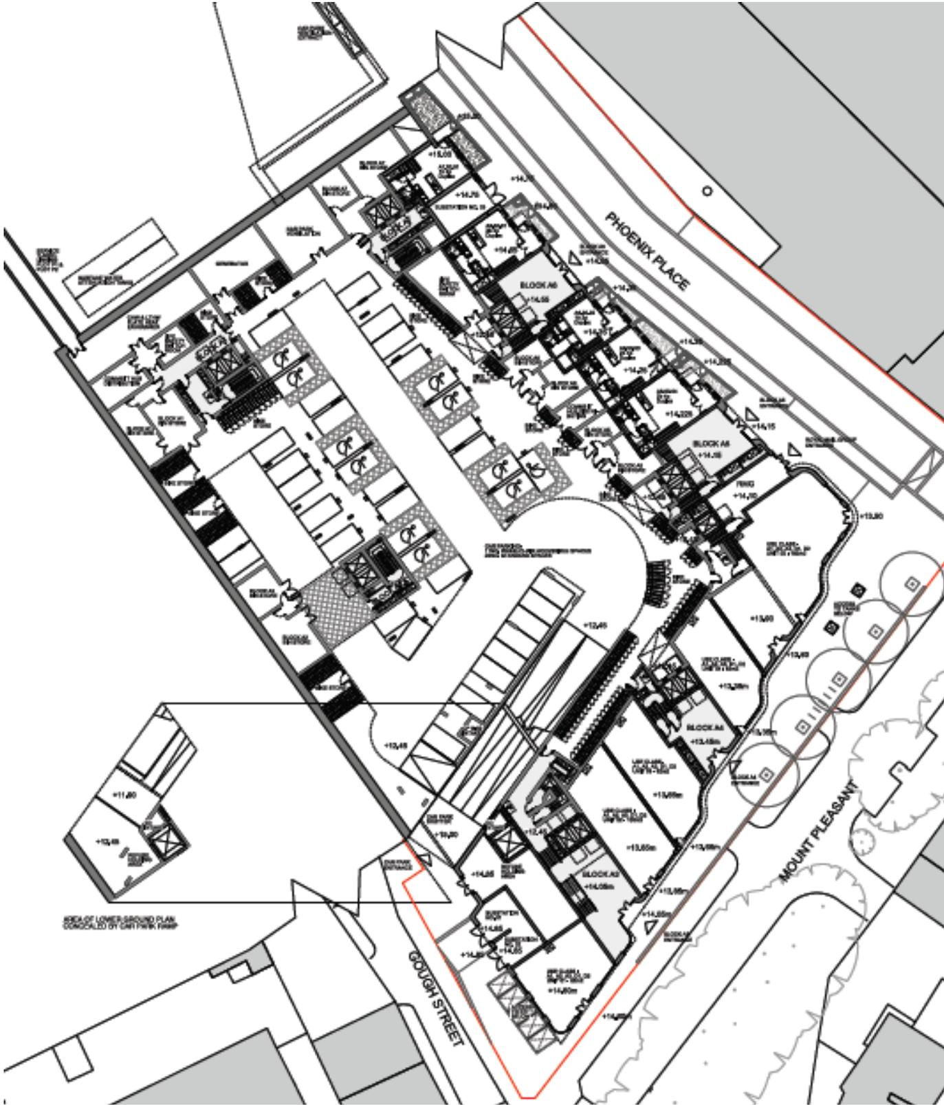
Full Camden site plan showing basement (north), ground floor (south west) and first floor (south east & east) levels, reflecting site topography
