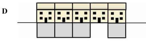
Multiple basement structures – adjoining basements
