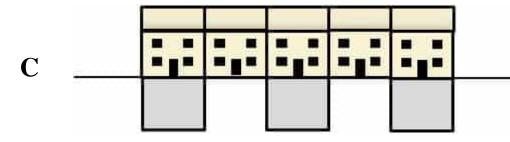
Multiple basement structures – no adjoining basements
