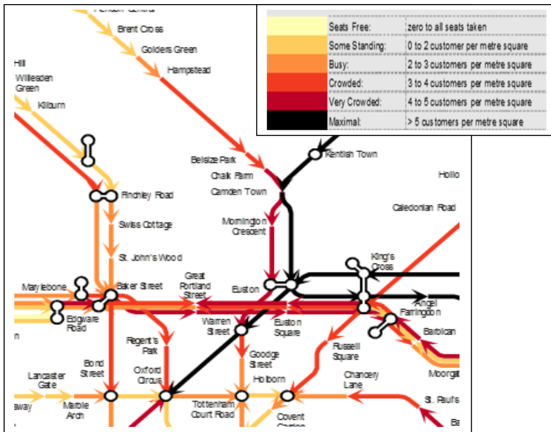
Figure 2.13: Tube network overcrowding in Camden by 2031 (weekday peak AM hour, includes planned investments)
