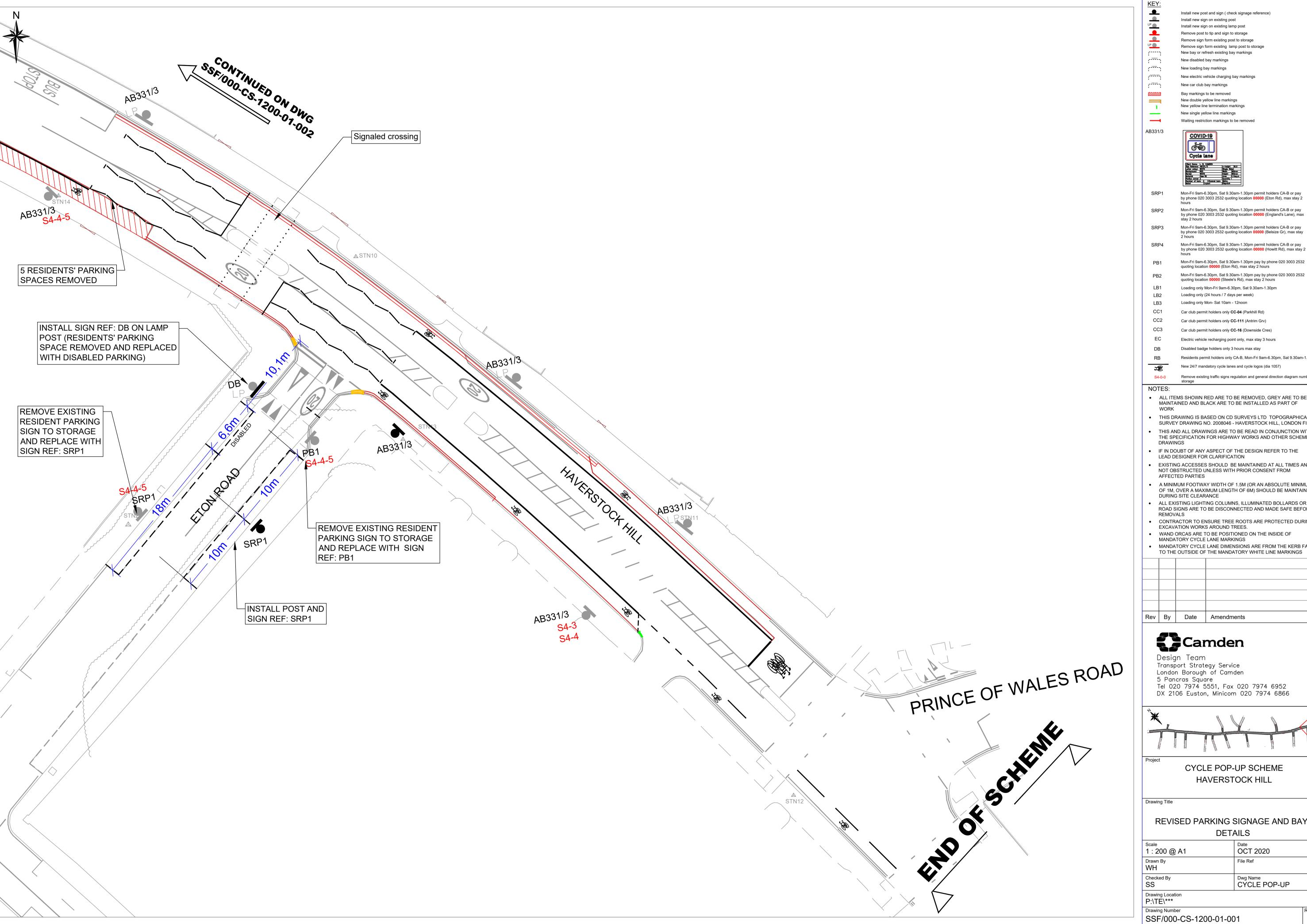
Install new post and sign ( check signage reference) Remove sign form existing post to storage Remove sign form existing lamp post to storage New bay or refresh existing bay markings New electric vehicle charging bay markings Waiting restriction markings to be removed
