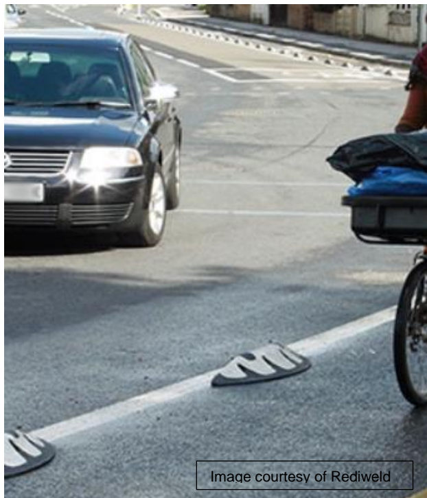
Image 4: 'Shared use bus boarder' (a raised section of cycle lane) placed at the bus stop, over which bus users have priority when boarding or alighting from a bus
