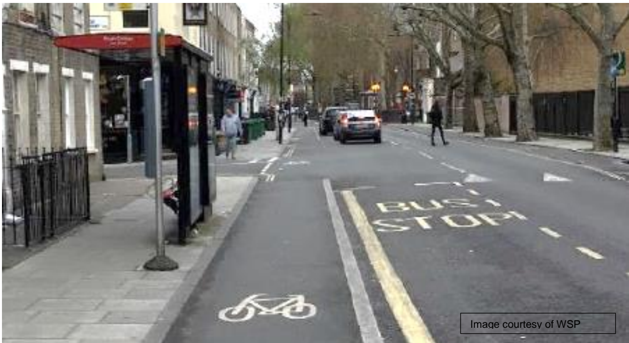
Image 4: 'Shared use bus boarder' (a raised section of cycle lane) placed at the bus stop, over which bus users have priority when boarding or alighting from a bus
